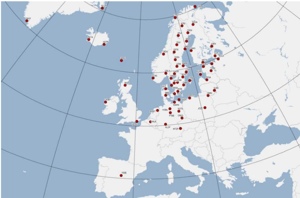
**Figure 1.1:** The NKG EPN LAC sub-network of 68 permanent reference stations for GNSS in January 2015. Source: [www.epncb.oma.be](http://www.epncb.oma.be).
