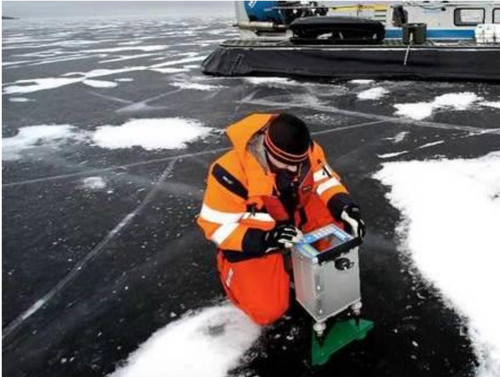
**Figure 1.8:** *Relative gravity measurements in March 2011 on Lake Vänern, the largest lake in Sweden. Photo: Mikael Lindblom.*
