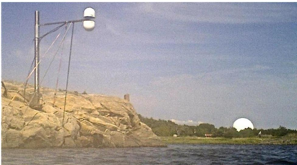
**Figure 2.3:** The GNSS tide gauge installation, with one zenith-looking and one nadir-looking antenna (covered by hemispherical radomes), at the Onsala Space Observatory. The radome of the 20 metre radio telescope in the background.
