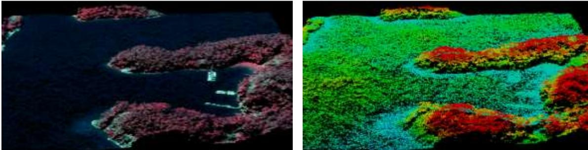
Figure 3: In the left image with IR colour, it is difficult to see that the matching has resulted in blurring over the water. It becomes clearer when the surface model is coloured based on elevation, like in the right image.
