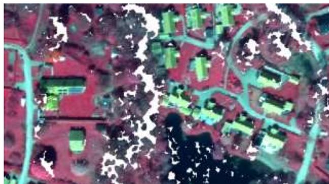
Figure 2: There will be holes in the digital surface model where matching has been unsuccessful. The holes can be clearly seen against a white background and can also be seen in the image on the front page of this document.
