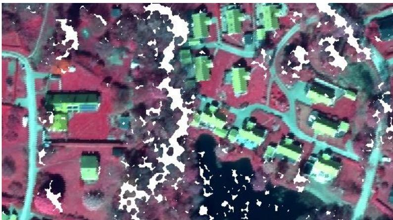
Matching does not work well on low-textured surfaces (surface patterns) as it is also difficult to find comparable points. Consequently, the surface model may be uneven for asphalted areas, certain fields etc. The surface model is to be used with caution for water areas. These may be uneven or include gaps as wave movements often cause the matching results to be blurry (see Figure 6 below).
