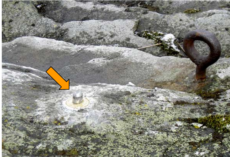
Figure 3. A 20 mm steel bolt anchored about 1 dm into the rock and used as monument in the local geodetic network.
