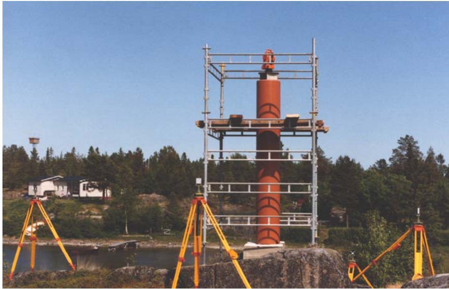
Figure 5. Picture from a SWEPOS station while establishing the local network. This pillar is not insulated. (The photo is from Sikskär – now SWEPOS station “Holmsund”, which was however not included in the original 21 SWEPOS stations.)
