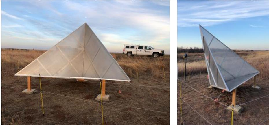
Artificial corner reflectors have been mostly in a passive form which functions as just signal reflectors without any electricity (see Figure 1) whereas recently the active ones (transponders, see Figure 2) have been developed and used in many experiments.
