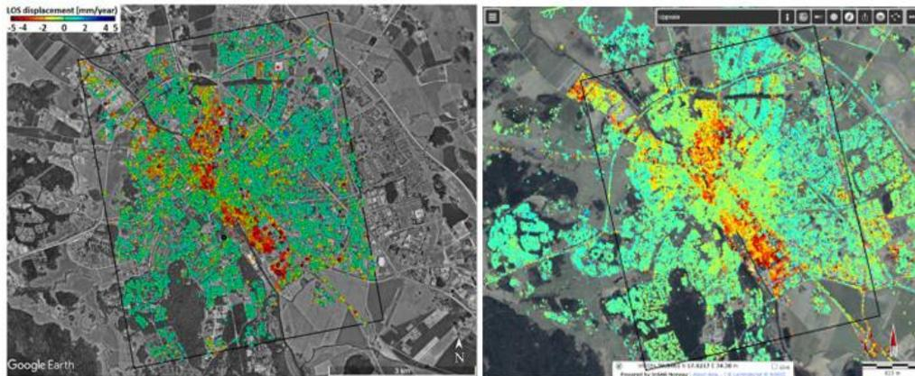
Figure 20, The LOS rate comparison between Uppsala and InSAR-Sweden.
