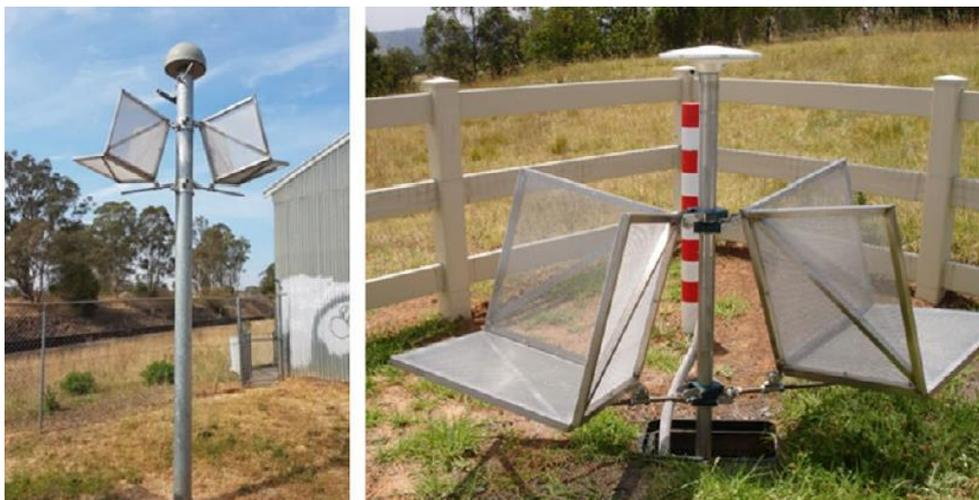
To investigate if our corner reflectors cause any multipath effect on nearby GNSS stations, we looked at the coordinate time series of the twin GNSS stations in two different locations, Sveg and Visby (see their locations in Figure 8). The installed corner reflector in Sveg is about 6 m away from the GNSS stations (see Figure 10) whereas, in Visby, the twin corner reflectors are about 20 metres away and have a different shape, size and orientation (see Figure 11).
