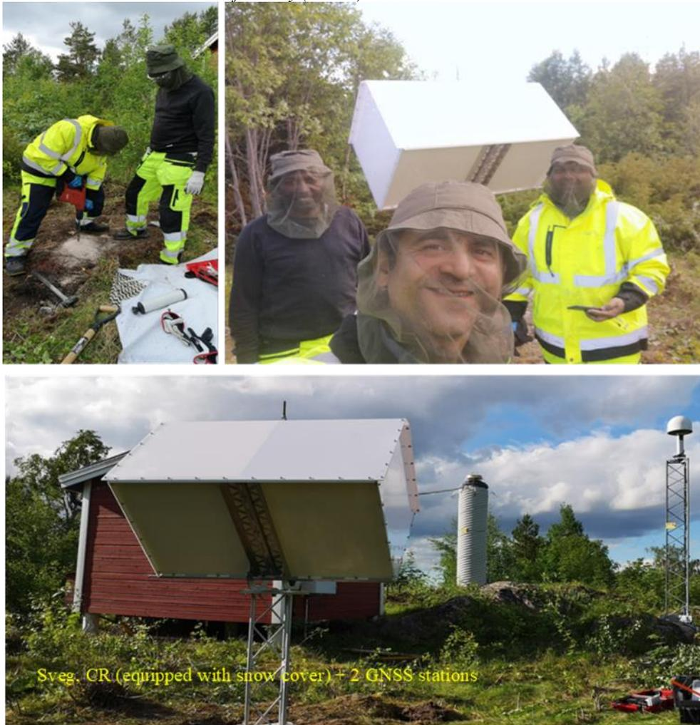
Figure 22, Different types of CRs installed at different locations (see Table 3 and Figure 8). Note the different shapes of the CRs and snow cover. The ones at Mårtsbo and Onsala are trihedral triangular types with inner leg of 1 metre and snow cover. The ones at Visby, are trihedral squared shape (trimmed version) with 1 m inner leg size, and snow cover. The ones at Östersund, Umeå and Skellefteå is double-backflipped squared shape with 72 cm inner leg and snow cover.
