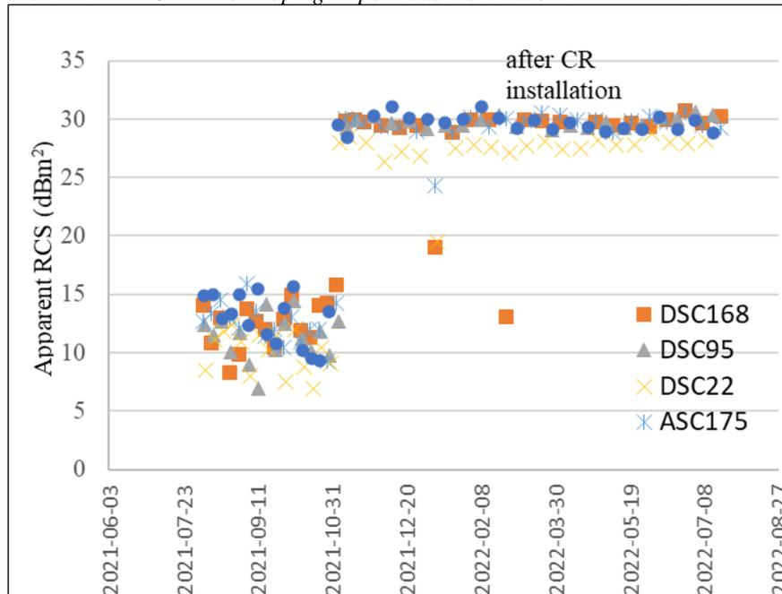
Figure 16, Estimated SCR values(dB) for corner reflector location using data for different Sentinel-1 tracks.
