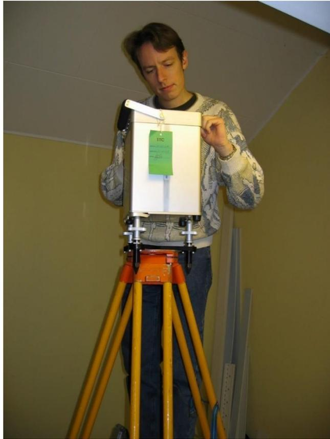
**Figure 55:** Gradient measurements at Onsala AS in 2007 with Scintrex CG5-198.
