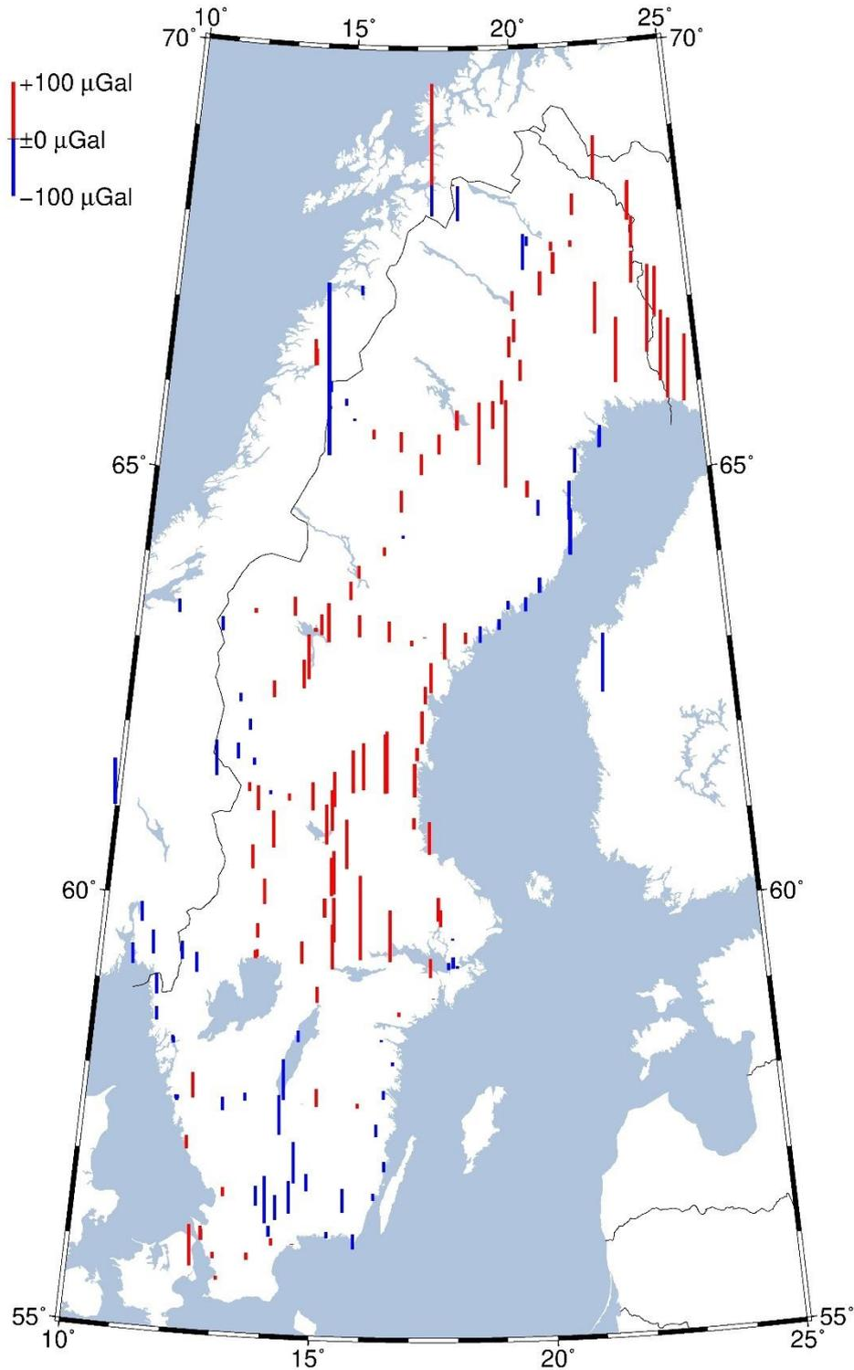
**Figure 79:** *Residuals in the two-step transformation between RG 62 and RG 2000 (2019 realization) after correction for land uplift for all RG 62 points.*
