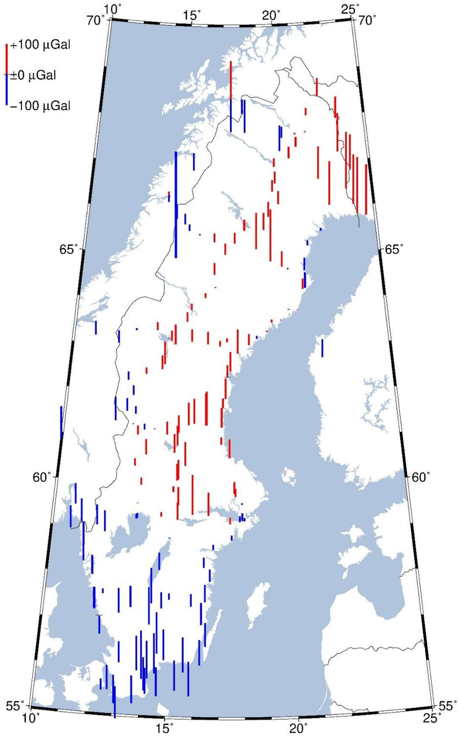
**Figure 80:** Compare to Figure 77. Residuals between RG 62 and RG 2000. The factor 14.68 mGal has been subtracted in order to get values to show in a figure.
