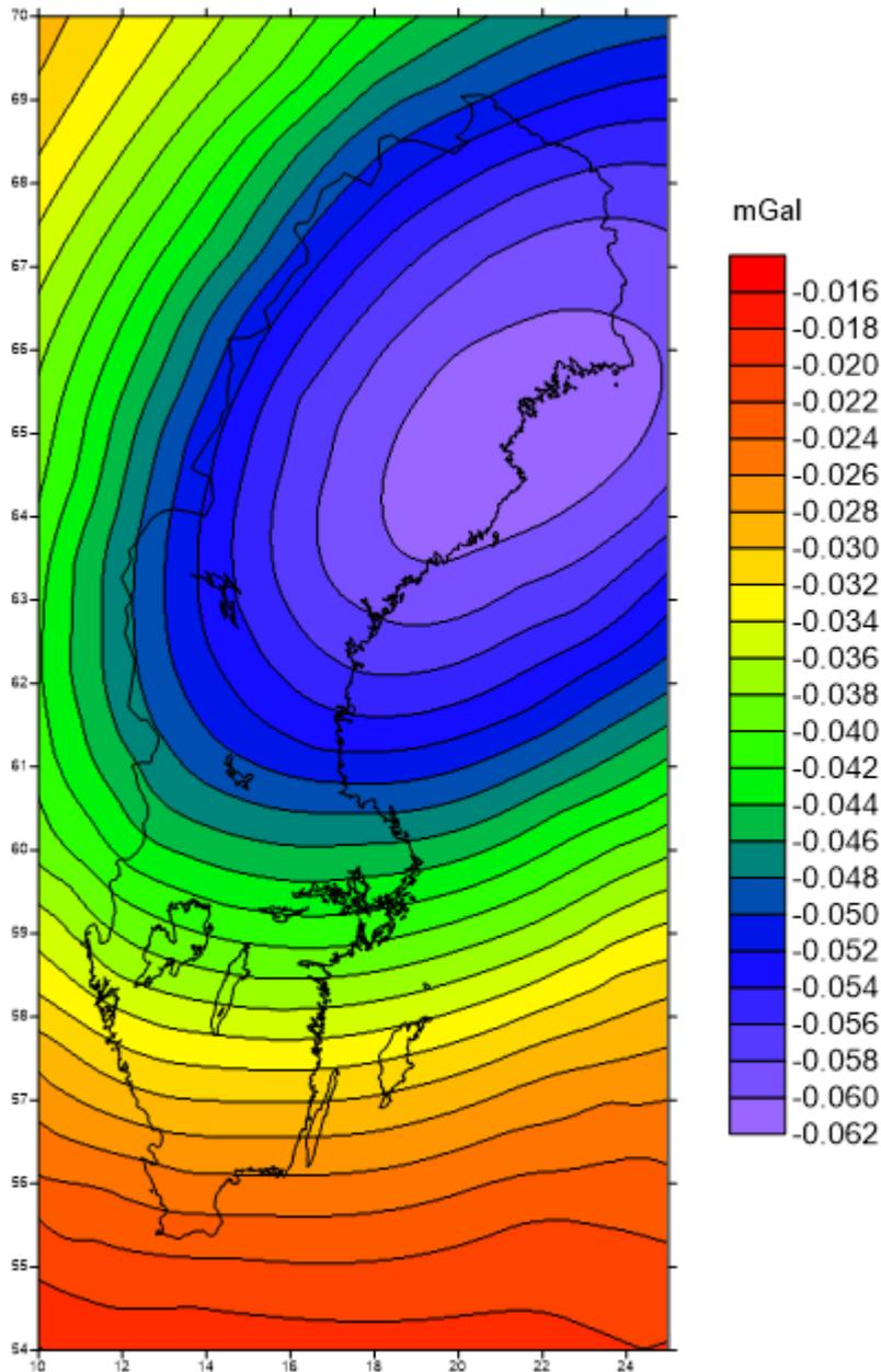
**Figure 74:** *The difference between RG 2000 and RG 82, the inclined plane transformation with the land uplift component included in the difference.*
