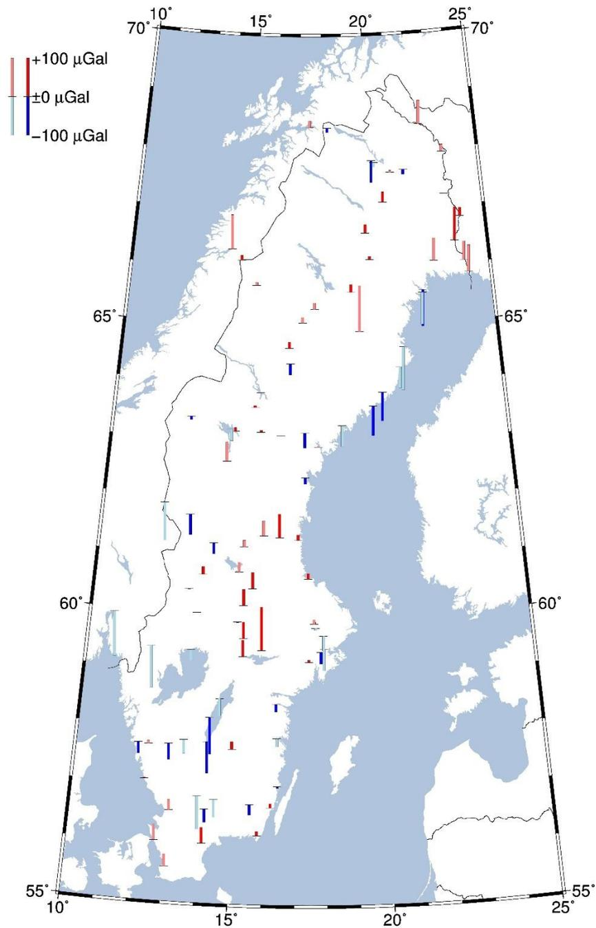
**Figure 76:** Residuals in the improved two-step transformation between RG 62 and RG 2000 after correction for land uplift. The darker blue and darker red points are the points used for the new transformation between RG 62 and RG 82. The lighter blue and lighter red points are the other check points, where we have connections between the systems.
