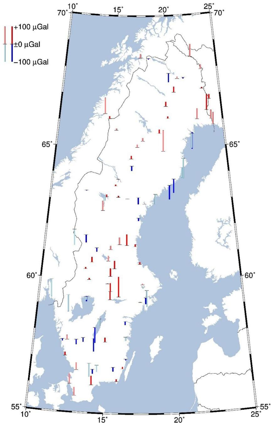
**Figure 78:** *Residuals in the transformation with the second-degree polynomial function between RG 62 and RG 2000 after correction for land uplift. The darker blue and darker red points are the points used for the transformation. The lighter blue and lighter red points are the other check points, where we have connections between the systems.*
