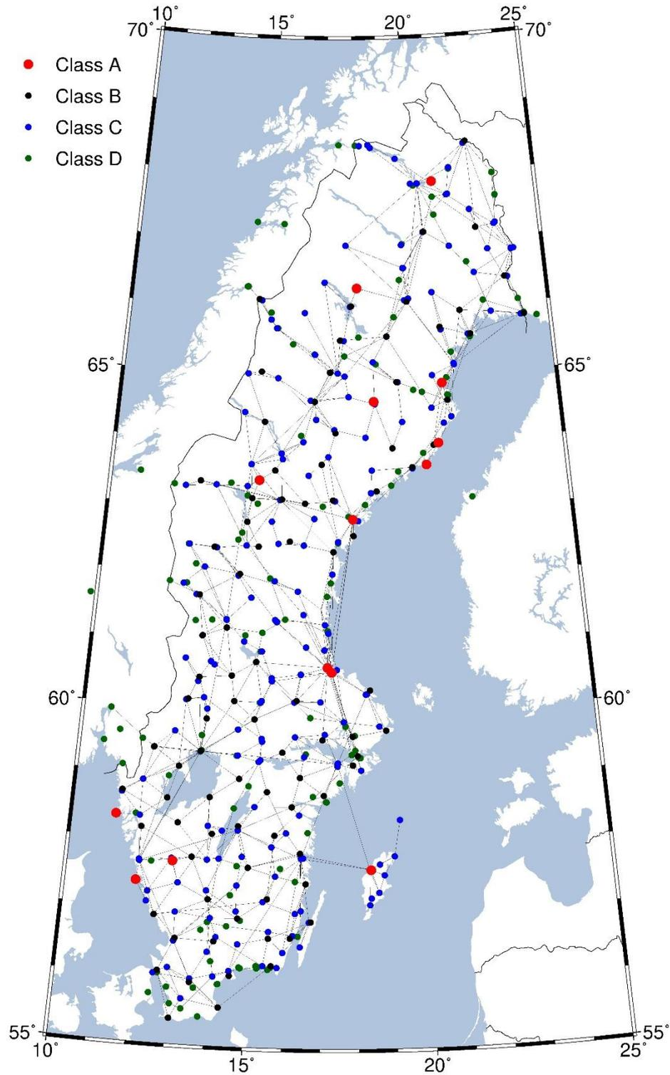
**Figure 1:** The RG 2000 gravity network. Red dots are Class A points, black dots Class B points, blue dots Class C points and green dots Class D points. The grey lines show how the Class A, B and C points are connected by relative gravity observations.
