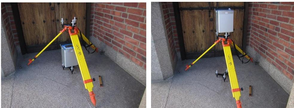
**Figure 56:** Gradient measurements at Östersund AB in 2013 with Scintrex CG5-740.
