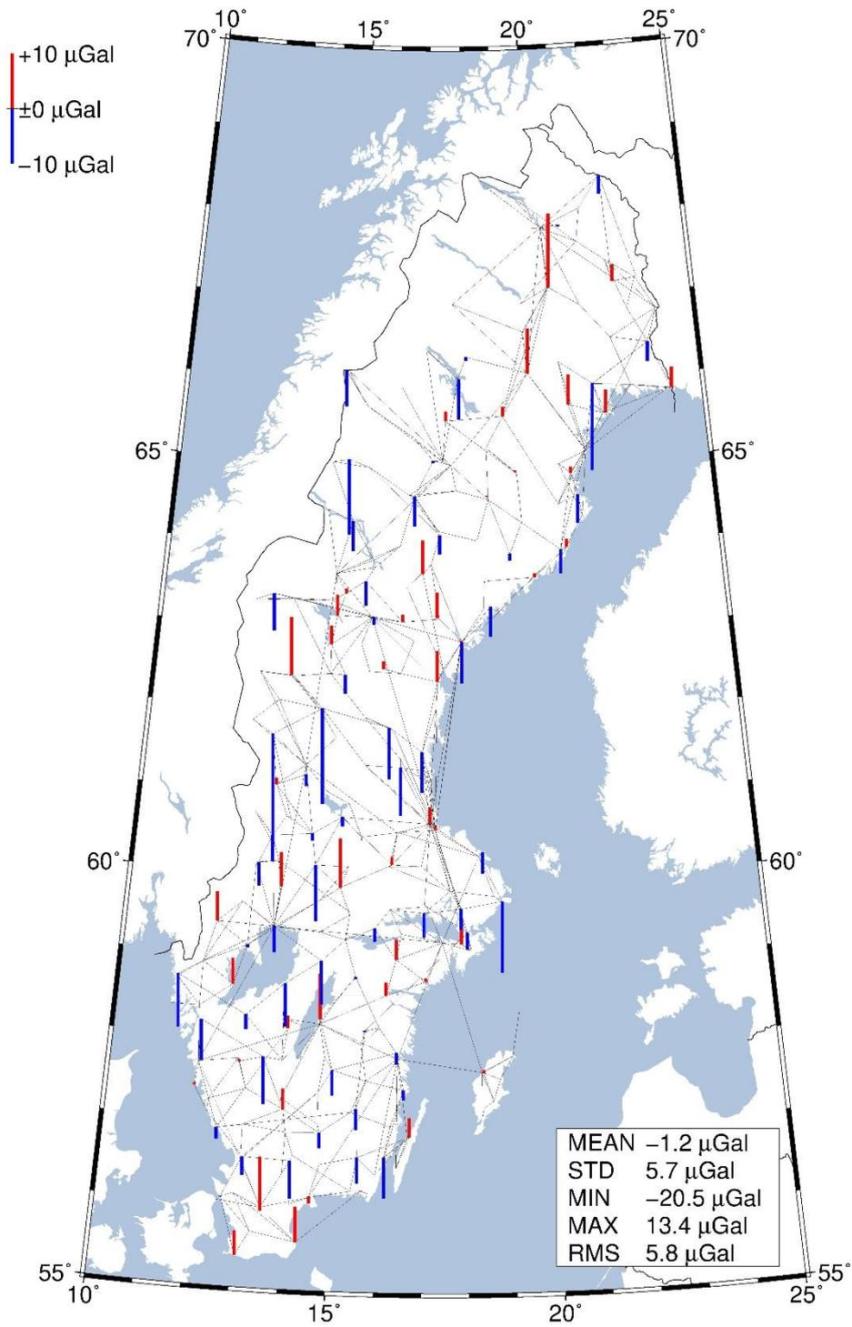
**Figure 63:** The residual of the results for the absolute observations. The larger the value, the more the value has changed in the adjustment.
