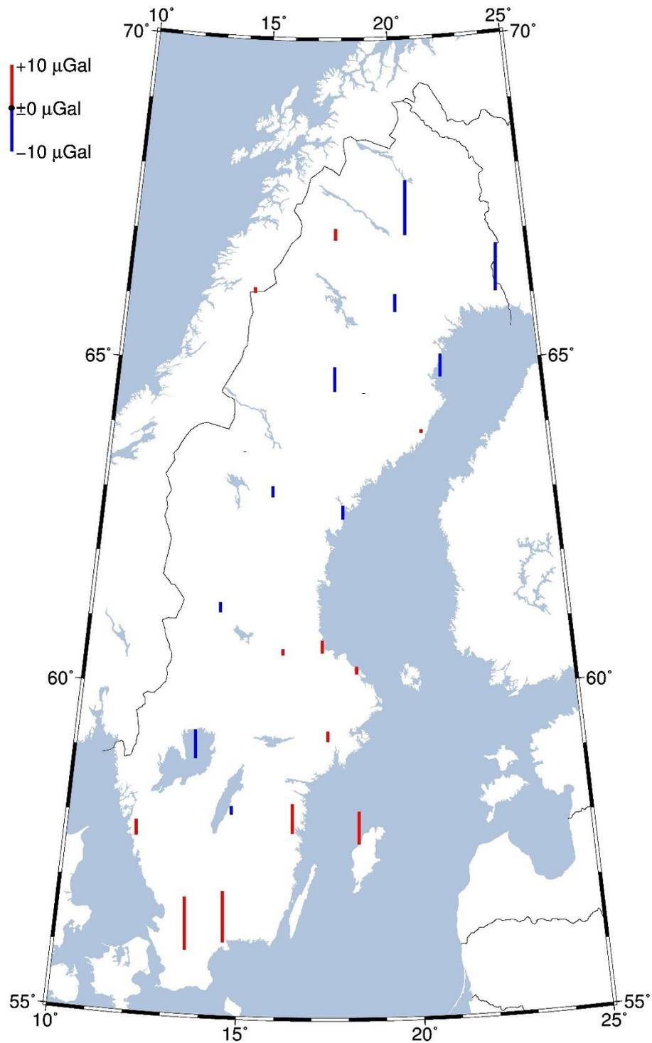
**Figure 71:** Residuals in 1-parameter fit between RG 2000 and RG 82 after correction for land uplift.
