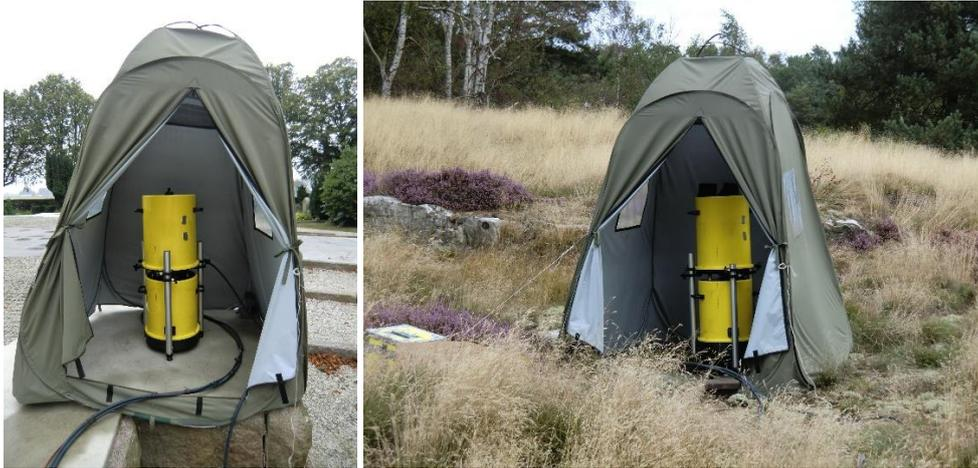
**Figure 33:** A10 observations at Maglarp AA (left, the point with the lowest  $g$ -value in RG 2000) and at Simrishamn AA (right).
