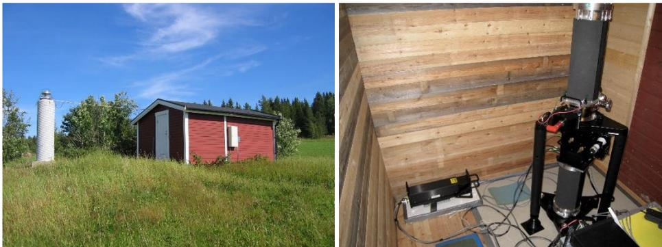
**Figure 13:** *Left: The building Östersund AA. Right: Observation with FG5-233 at Östersund AA in 2008.*
