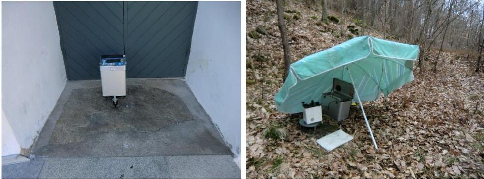
**Figure 48:** Observations in 2013, at Grinneröd AA with CG5-740 (left) and at Veddige with G54 (right).
