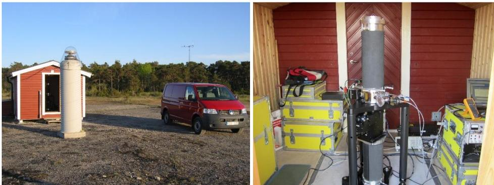
**Figure 15:** *Left: The building Visby AA. Right: Observation with FG5-233 at Visby AA in 2011.*
