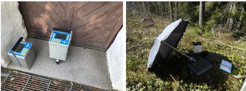
**Figure 49:** Observations at the two original end points of the calibration line, Husby-Ärlinghundra AA with Scintrex CG5-1184 and with Scintrex CG5-740 standing on the left side waiting for its turn in 2019 (left) and Boda Bruk AA with LCR G54 in 2016 (right, even if this particular photo shows an observation for RG 2000).
