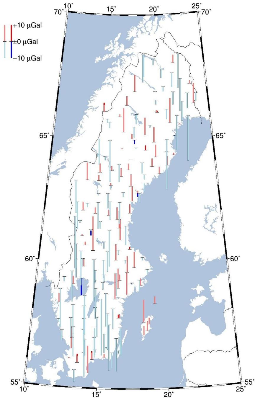
**Figure 73:** Residuals in the inclined plane transformation between RG 82 and RG 2000 after correction for land uplift, for 200 points. Some larger errors in RG 82 can be found.
