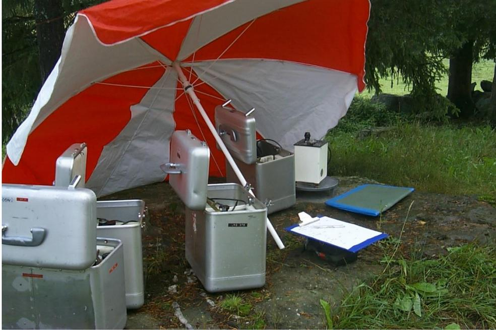
**Figure 5:** Observations in Joensuu (Finland) along the 63<sup>rd</sup> degree line in 2003 with two Swedish (G54 and G290) and two Norwegian (G45 and G378) gravimeters.
