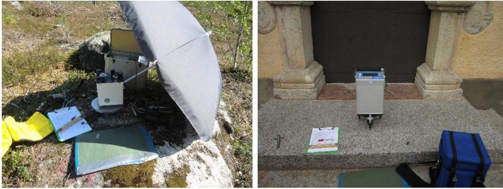
**Figure 43:** Observations for RG 2000 in 2016, at Hoting with LCR G54 (left) and at Leksand AA with CG5-1184 (right).
