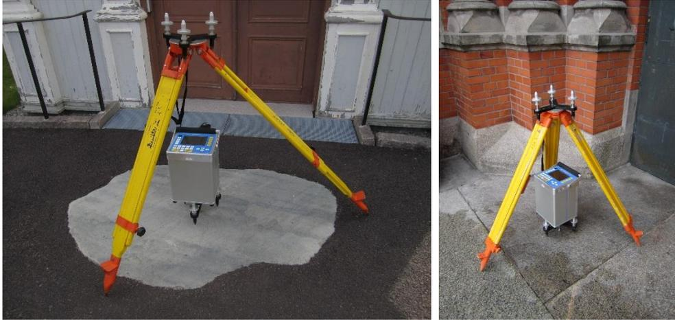
**Figure 47:** *Gradient measurements with Scintrex CG5-740 at Hede AA in 2012 (left) and at Luleå AA in 2013 (right).*
