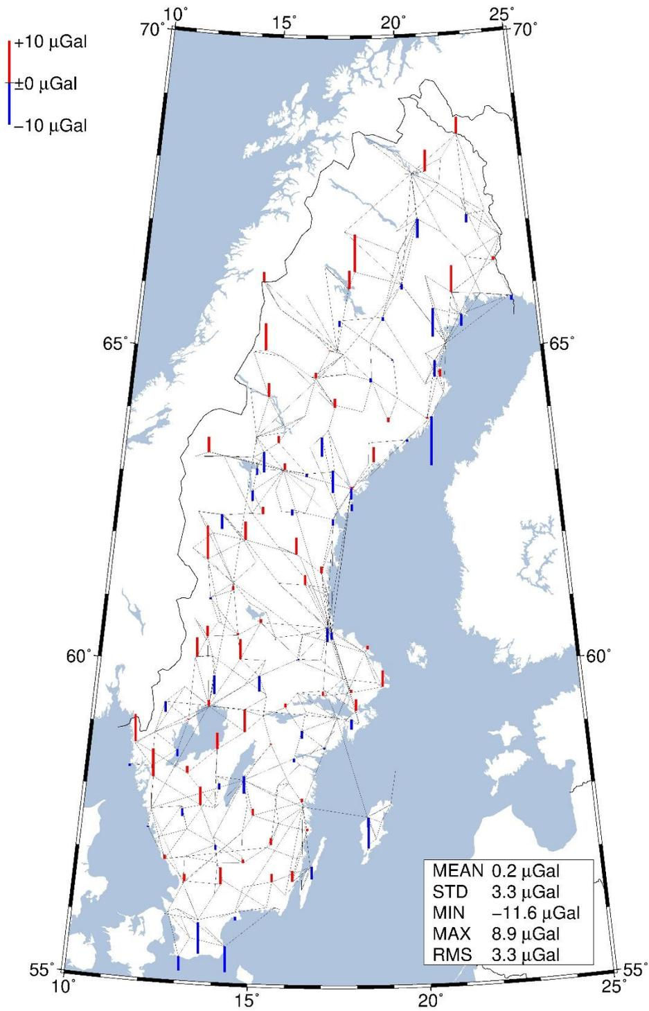
**Figure 65:** *The difference between the adjusted result and the leave-one-out cross validation. The larger the value, the less the absolute gravity observation and the relative gravity observations correspond to each other.*
