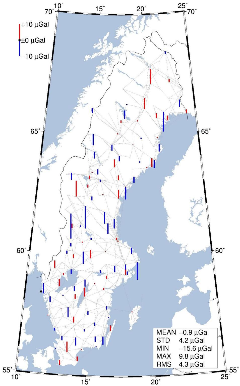
**Figure 59:** The residual of the results for the absolute observations. The larger the value, the more the value has changed in the adjustment.
