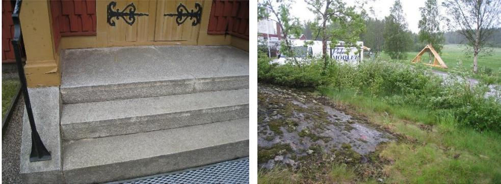
**Figure 23:** Photos from the reconnoitering. Left: Ljusnarsberg AA, an RG 62 point which fitted perfectly for A10 observations. Right: Lövånger, an RG 82 First Order point which surface is leaning too much for an A10 and even for a relative gravimeter.
