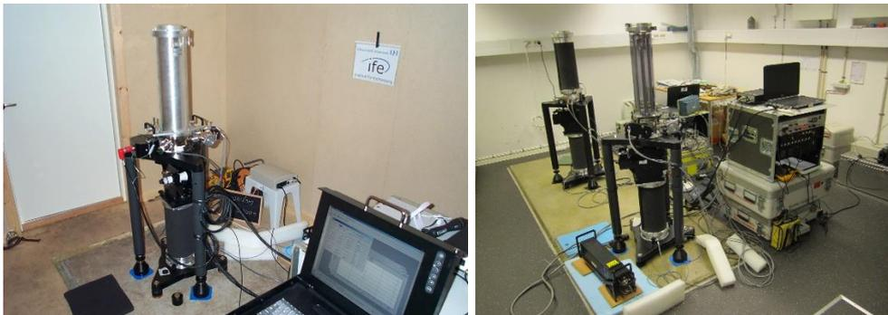
**Figure 27:** FG5-220 observation in Kramfors AA (left, in 2004) and comparison between FG5-233 and FG5X-220 in Onsala AA/AC (right, in 2014).
