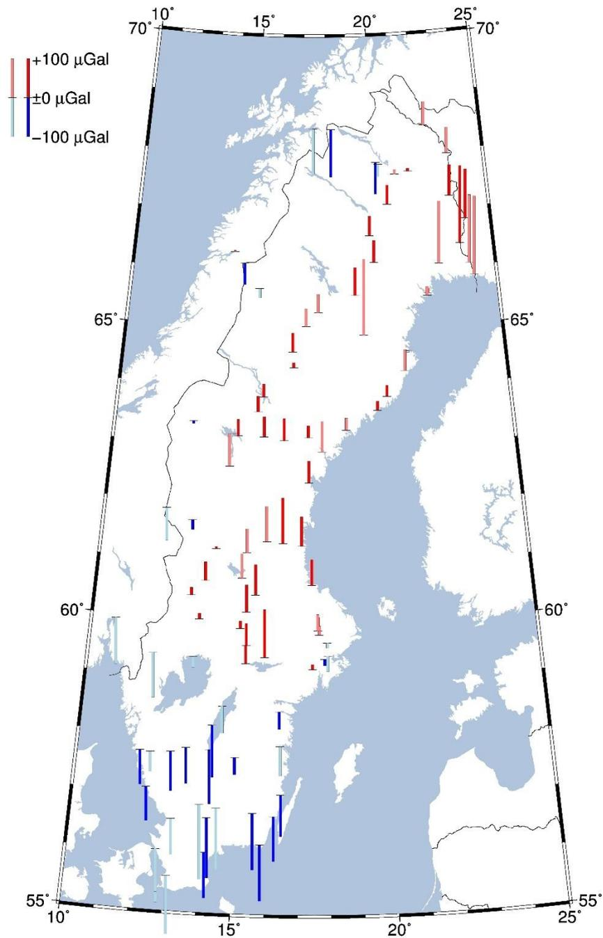
**Figure 77:** Residuals in the 1-parameter transformation between RG 62 and RG 2000 after correction for land uplift. The darker blue and darker red points are the points used for the transformation. The lighter blue and lighter red points are the other check points, where we have connections between the systems.
