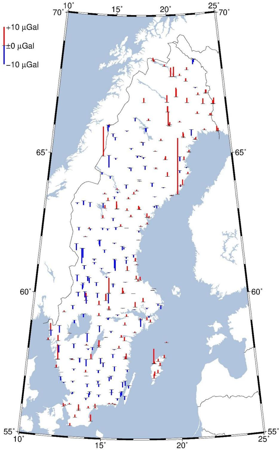
**Figure 66:** *The difference between the RG 2000 realization from 2018 and the new RG 2000 realization from 2019 (old-new), only for the points included in both the main adjustments.*
