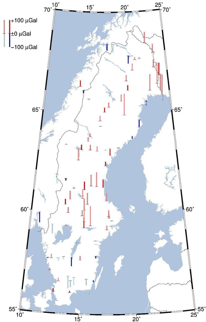
**Figure 75:** Residuals in the two-step transformation between RG 62 and RG 2000 after correction for land uplift. The darker blue and darker red points are the points used for the old transformation between RG 62 and RG 82. The lighter blue and lighter red points are the other check points, where we have connections between the systems.
