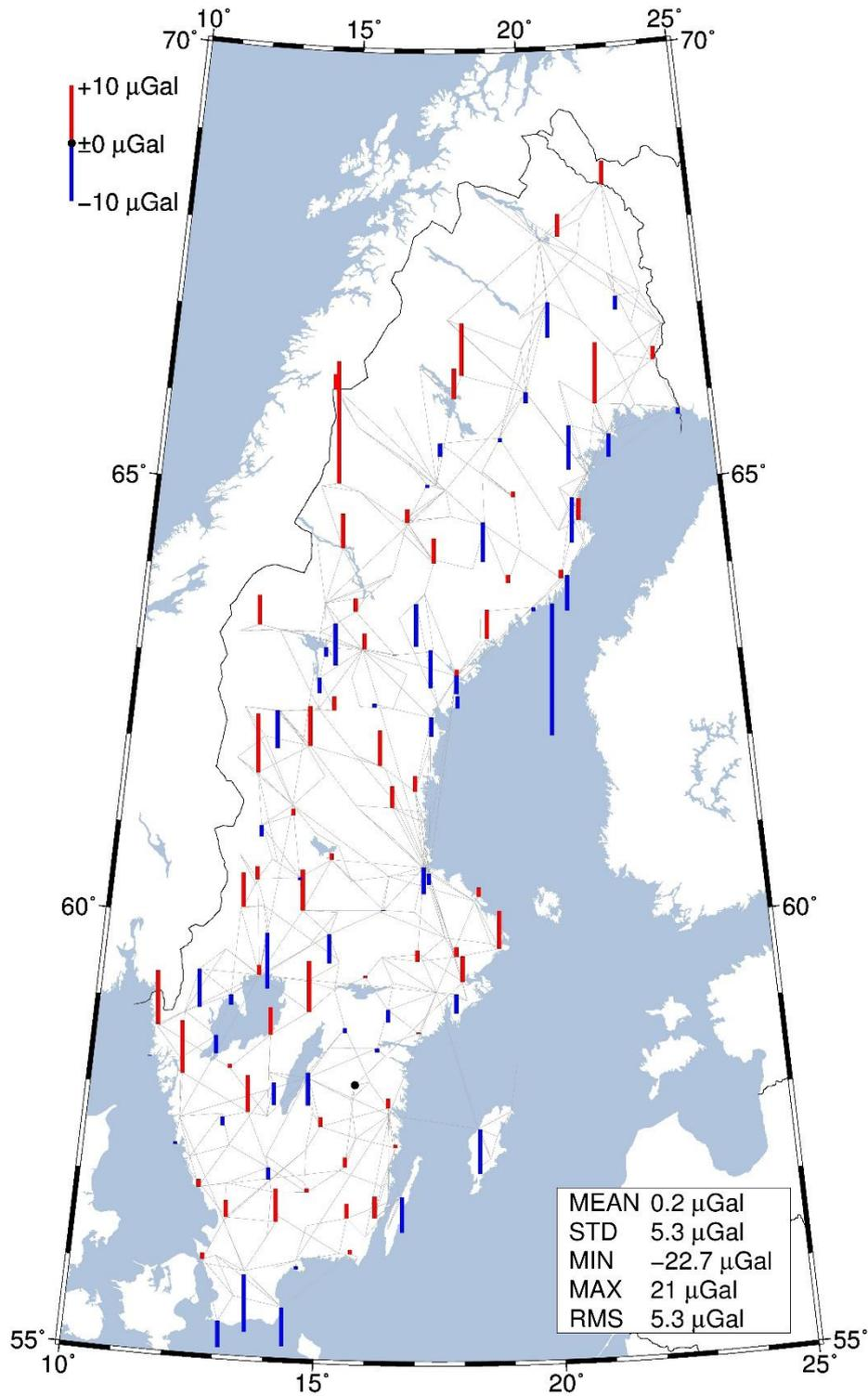
**Figure 61:** *The difference between the adjusted result and the leave-one-out cross validation. The larger the value, the less the absolute gravity observation and the relative gravity observations correspond to each other.*
