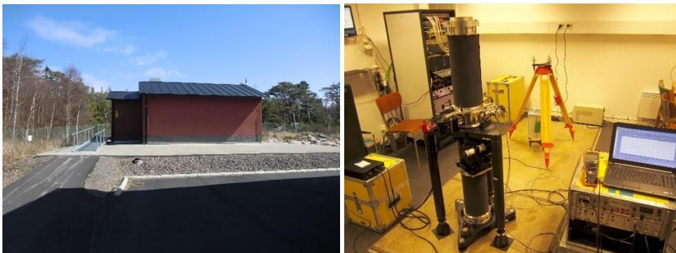
**Figure 8:** *Left: The new gravimeter building in Onsala. Right: FG5-233 observing at Onsala AA in 2015, the Scintrex relative gravimeter is standing at Onsala AC.*
