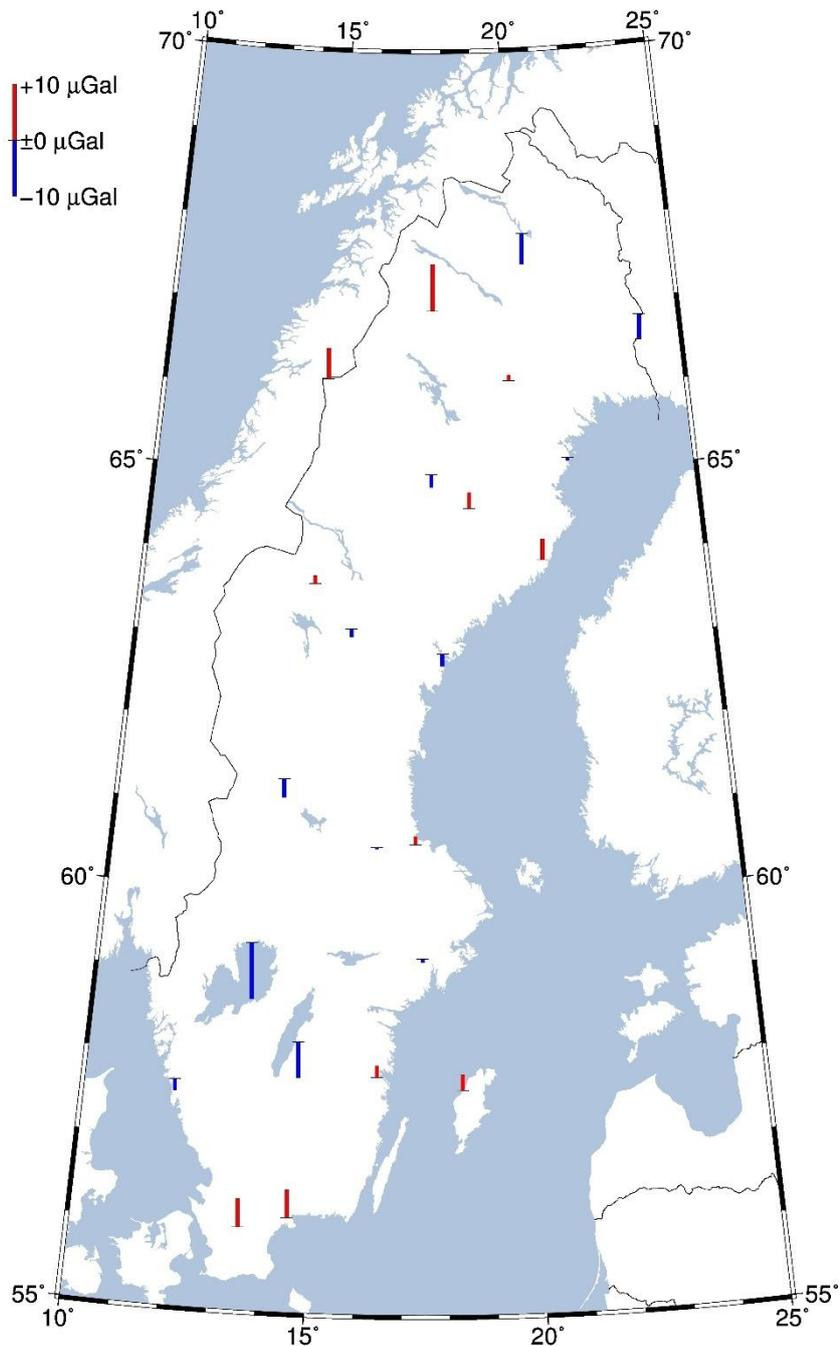
**Figure 72:** Residuals in the inclined plane transformation between RG 82 and RG 2000 after correction for land uplift.
