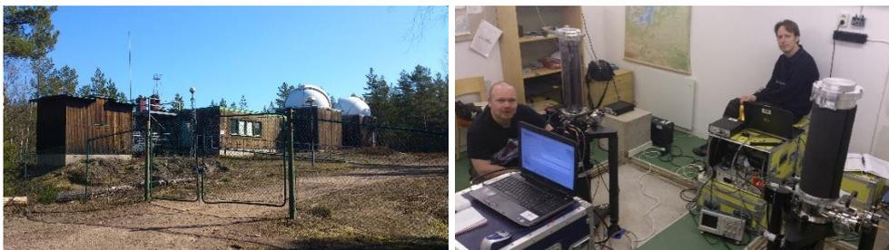
**Figure 7:** Left: Mårtsbo, the building. Right: Comparison in Mårtsbo in 2015. FG5-233 is at Mårtsbo AA (right, next to Andreas Engfeldt) and FG5X-221 (FGI) is at Mårtsbo AB (left, next to Jyri Näränen).
