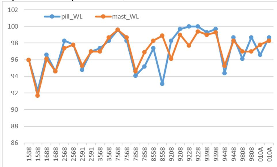
**Figure 4:** Narrow lane (NL) ambiguity resolutions (in %) for each 24 hours session (including only 1 unknown point (shown in horizontal axis) and 5-8 reference mast or pillar stations).
