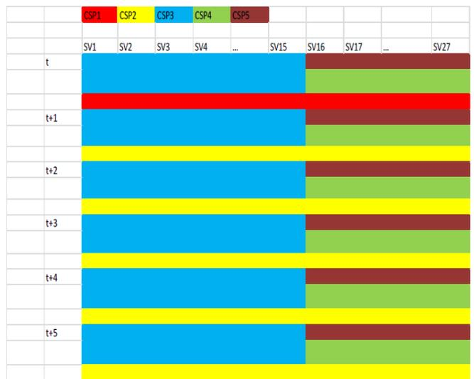
Fig. 3. Potential breakup of the service provision within a multi-second signal.
