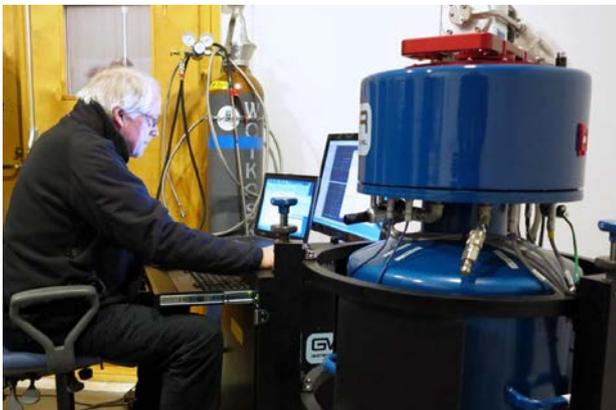
**Fig. 10.** Installation of the new superconducting gravimeter at Metsähovi. Photo M. Poutanen
