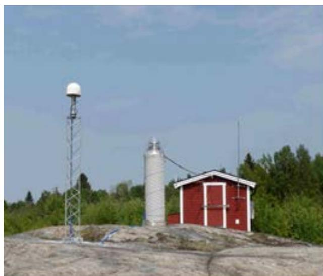
**Fig. 1.3.** *Hässleholm is one of the SWEPOS stations belonging to class A. It has both a new monument (established in 2011) and an old monument (from 1993).*
