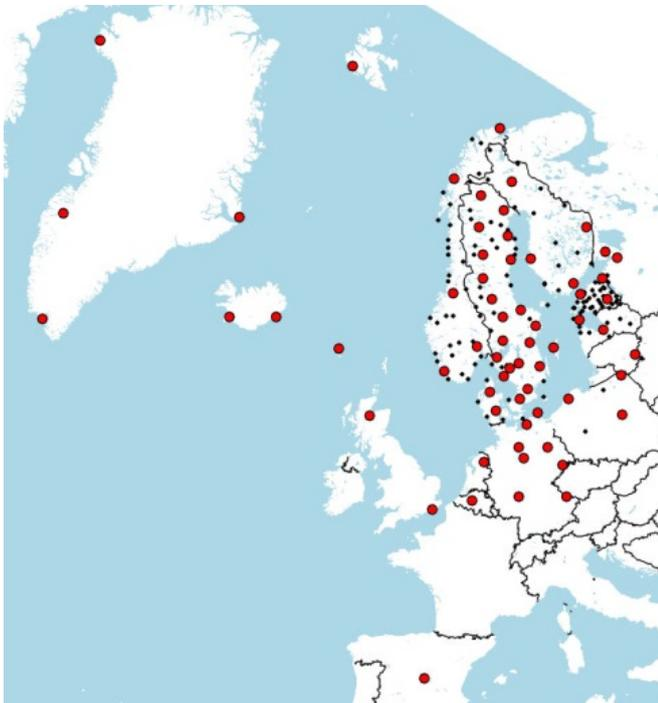
**Fig. 2:** The combined network of NKG GNSS AC, Nov. 2014. Red dots are stations included in the NKG EPN-solution and the black dots are national stations.
