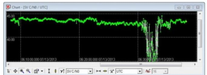
**Fig. 2.** The variation of the signal-to-noise [dBHz] averaged over all tracked satellite signals for one of the detected incidents. The first two thirds of the time series shows normal variation. The interference signal is active during the last third of the plot.
