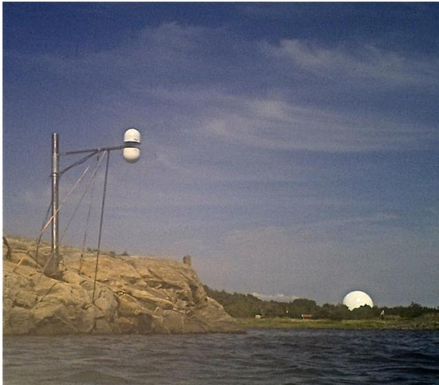
**Fig. 2.3.** *The GNSS tide gauge installation, with one zenith-looking and one nadir-looking antenna (covered by hemispherical radomes), at Onsala Space Observatory. The radome of the 20 metre radio telescope in the background.*
