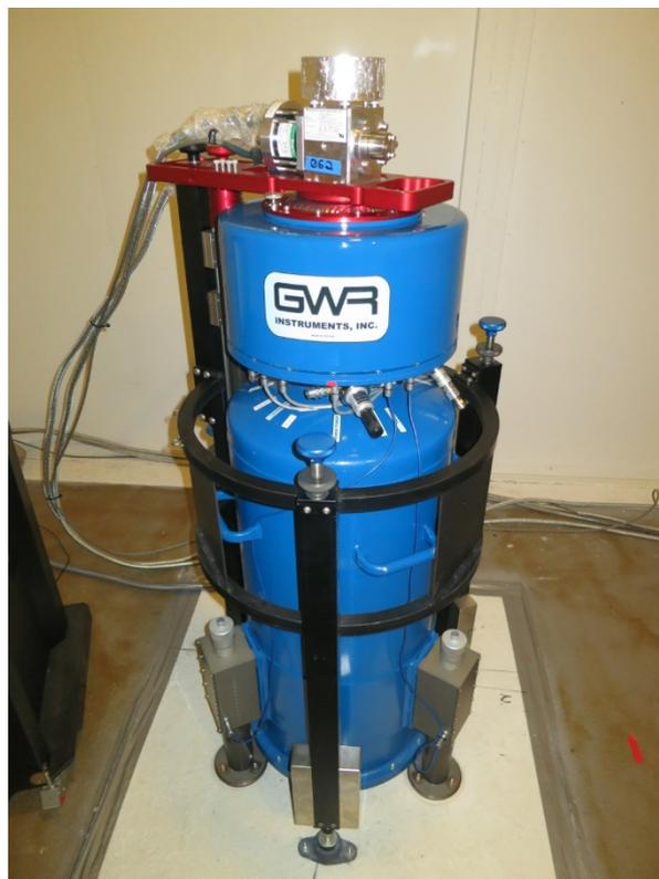
**Fig. 6.** New superconducting gravimeter OSG-073 of the FGI. Photo J. Näränen
