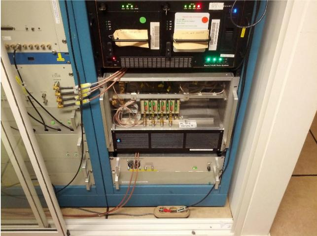
**Fig. 2.1.** The new rack for VLBI at Onsala Space Observatory is a modern digital backend system.
