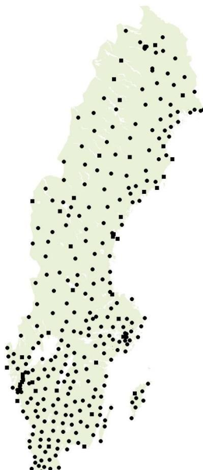
Figure 1: The SWEPOS network in May 2013. Squares indicate class A stations and dots indicate class B stations.
