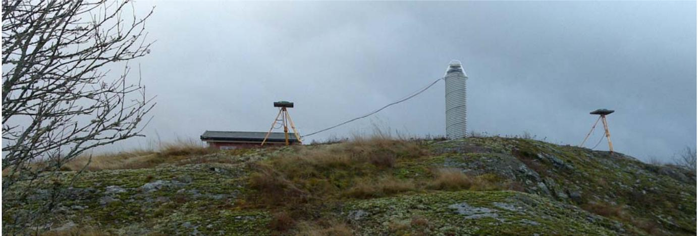
**Fig. 3.** Vänersborg, 2009. SWEPOS antenna monument, together with two benchmark setups. The SWEPOS equipment cabin can be seen in the background.
