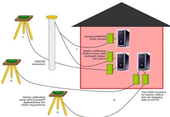
**Fig. 1.** Principle sketch of the station calibration setup.
