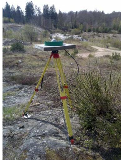
**Fig. 2.** Hässleholm, 2010. One of the bench–mark setups. An Eccosorb plate is mounted directly beneath the choke-ring antenna. The GNSS receiver is kept in the SWEPOS equipment cabin during the campaign.
