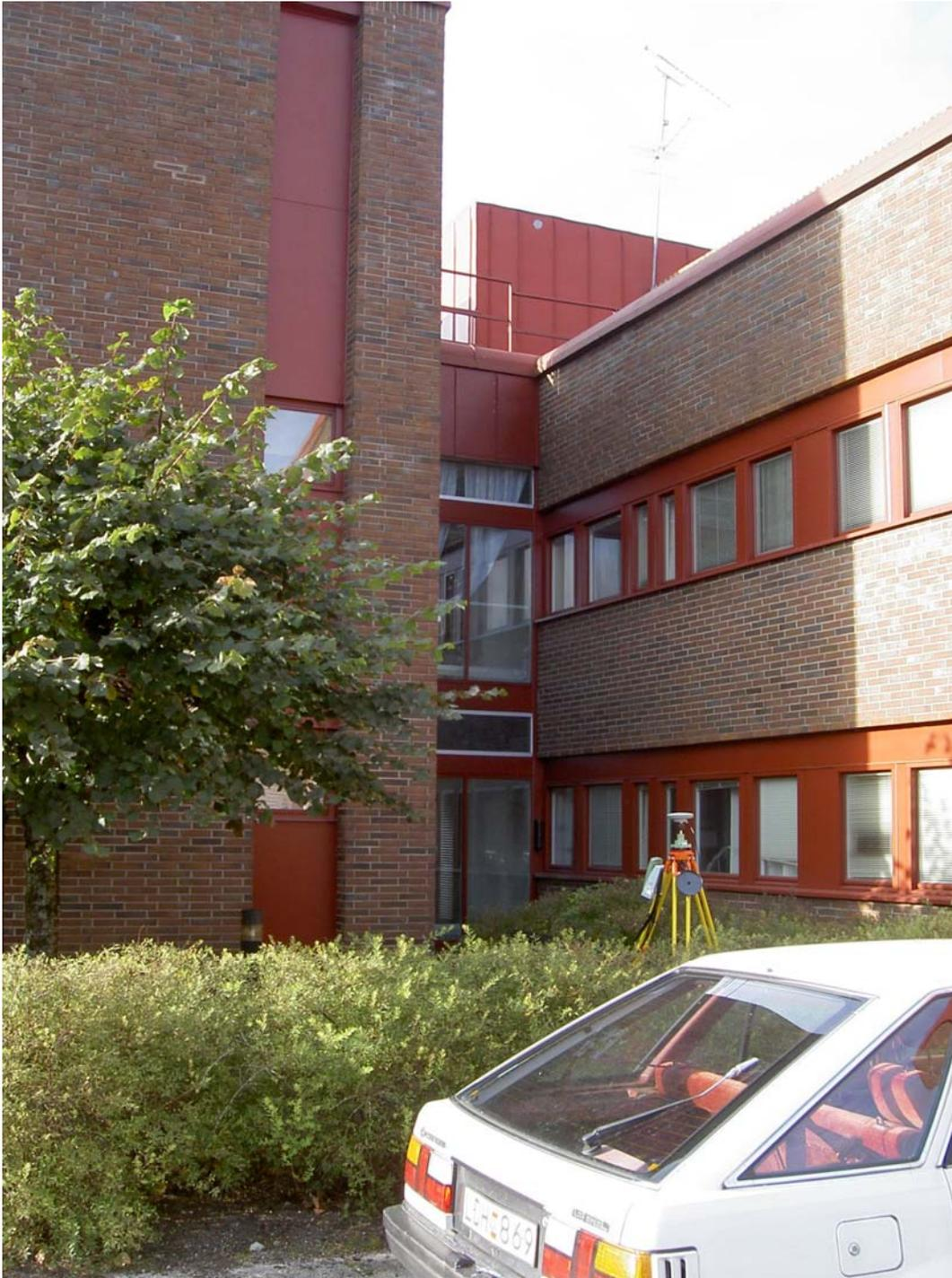
**Figure 17** Antenna setup for the characterization of signal multipath in a difficult environment.
