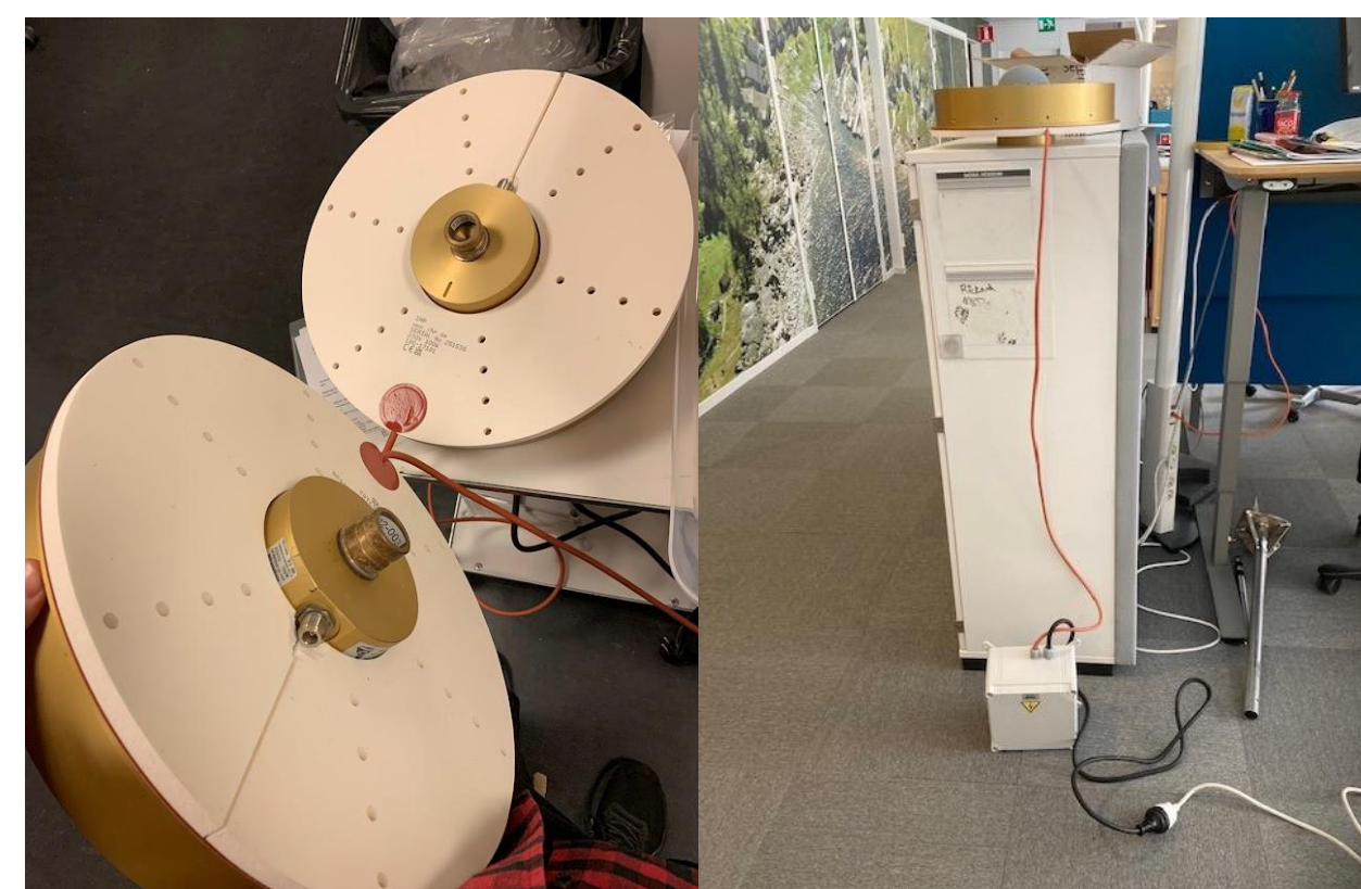
Figure 6. New antenna heaters.
