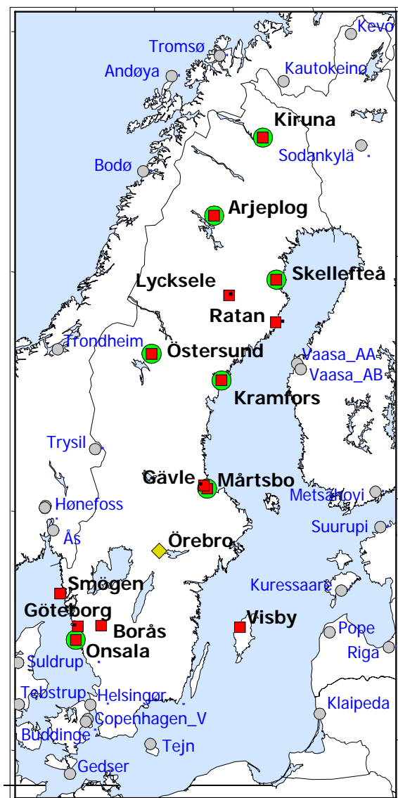
2 Figure 5: Absolute gravity sites in Sweden (red squares), planned new site (yellow diamond) and sites in neighbouring countries (grey circles). Sites 2 observed every year since 2003 have a green circle as background to the red square.
