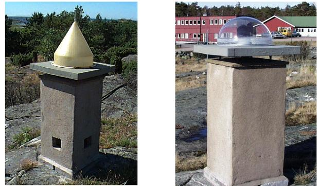
Figure 7: GPS antenna with radome at Onsala before and after February 1, 1999.
