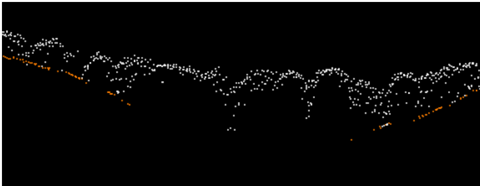
Figure 3. Due to the dense vegetation, no laser points have reached the ground in the depression. The classification was accurate, but there is a shortage of ground points. When the terrain model is created, this surface will be interpolated. White points are unclassified, orange points are ground.
