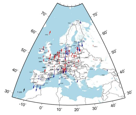
*Figure 8: ITRF2014, epoch 2015.5 to ETRF2000 epoch 2007, vertical residuals in the Helmert-transformation. Red arrows are positive residuals and blue are negative.*
