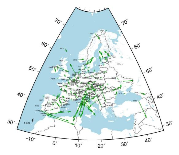
Figure 9 : ITRF2014, epoch 2022.5 to ETRF2000 epoch 2007, horizontal residuals in the Helmert-transformation.
