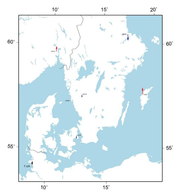
Figure 18: ITRF2014, epoch 2022.5 to SWEREF 99, vertical residuals in the Helmert-transformation.
