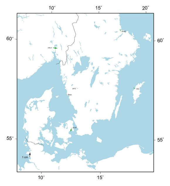
Figure 15: ITRF2014, epoch 2015.5 to SWEREF 99, horizontal residuals in the Helmert-transformation.
