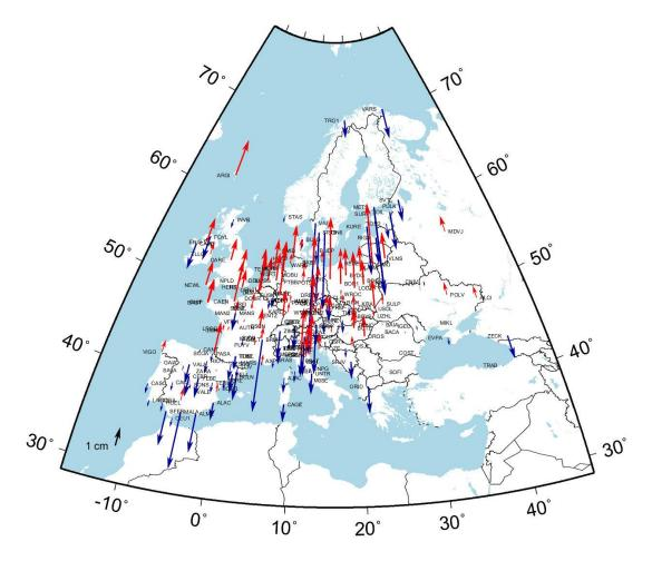
Figure 10: ITRF2014, epoch 2022.5 to ETRF2000 epoch 2007, vertical residuals in the Helmert-transformation.
