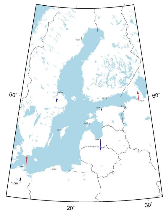
Figure 12: ITRF2014, epoch 2015.5 to ETRF97 epoch 1998.5, vertical residuals in the Helmert-transformation.
