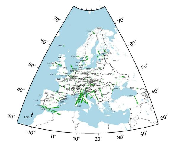
Figure 7: ITRF2014, epoch 2015.5 to ETRF2000 epoch 2007, horizontal residuals in the Helmerttransformation.
