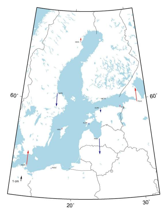
Figure 14: ITRF2014, epoch 2022.5 to ETRF97 epoch 1998.5, vertical residuals in the Helmert-transformation.
