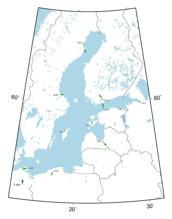
Figure 13: ITRF2014, epoch 2022.5 to ETRF97 epoch 1998.5, horizontal residuals in the Helmert-transformation.
