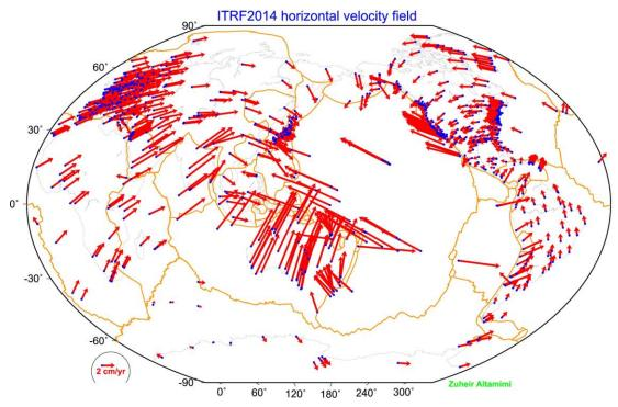
Figure 1: The plate tectonics described by the ITRF2014 velocity field [Altamimi et. al. 2016].
