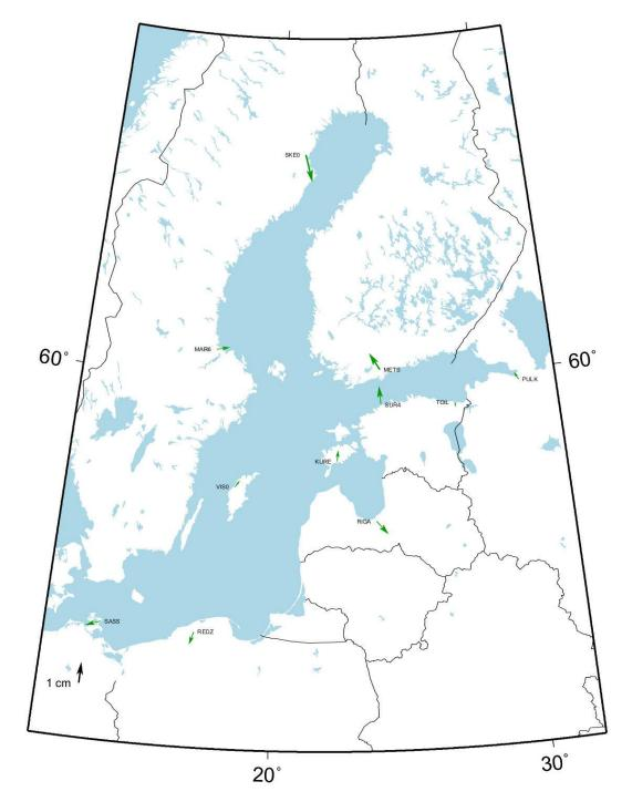
Figure 11: ITRF2014, epoch 2015.5 to ETRF97 epoch 1998.5, horizontal residuals in the Helmerttransformation.
