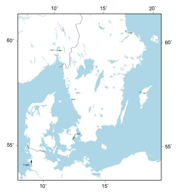
*Figure 17: ITRF2014, epoch 2022.5 to SWEREF 99, horizontal residuals in the Helmert-transformation.*
