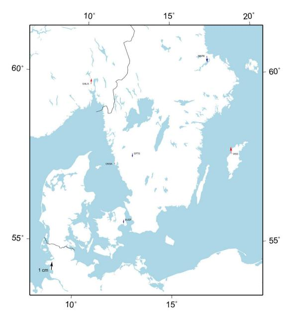
Figure 16: ITRF2014, epoch 2015.5 to SWEREF 99, vertical residuals in the Helmert-transformation.
