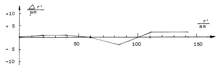
Distortion on the semidiagonals related to the symmetry point of distortion
