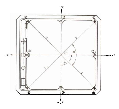
K  $\triangleq$  Temperature difference t - t<sub>0</sub>, with t<sub>0</sub> = 22° C. M'= Centre of fiducial mark (intersection point of the fiducial mark connecting lines in the centre of the format sides) = zero point of image coordinate system.
